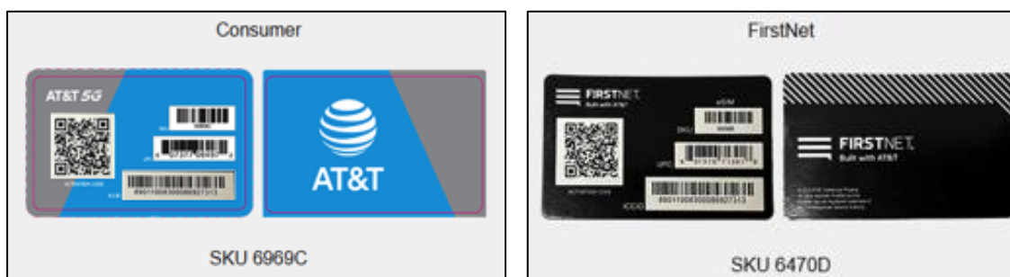
Figure 4 – Examples of physical eSIM cards from AT&T and FirstNet.
