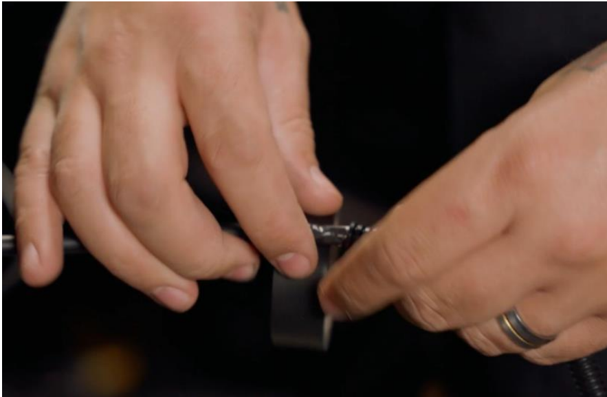
Figure 7 – Protecting the cables with tape.
