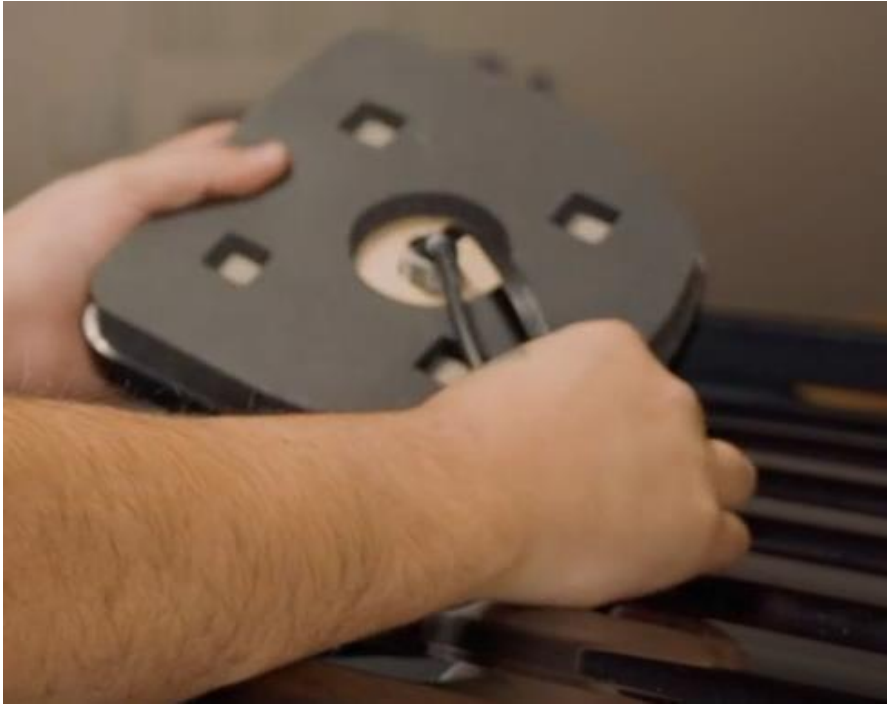
Figure 11 – Routing the cables through the hole.
