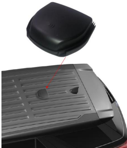
Figure 3 – Installing AC-Fleet on top of a rib..
